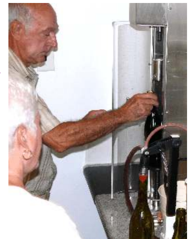
A bottling station, (the wine station has four) all with automatic corkers.
